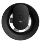
Pax Norte black 1561-1 Yes 110 m3/h 30 25Pa 4W 17-20 dB(A) 3 m 100-240V AC 50/60Hz / or 12V DC EC BTLE4 IP44 Class II (does not require earth protection) S-Intertek CE Ø100-140 mm 5-35 Qualified installation engineer 0.38
