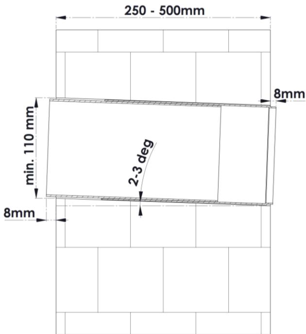
For the installation of BSK Zephyr Mini decentralized heat recovery device, a hole must be drilled on a wall facing the exterior with the dimensions indicated in the figure.
