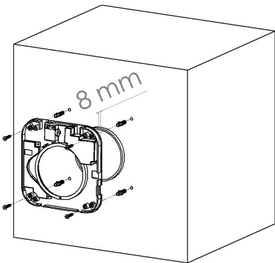
1. Align the inner wall fixture part with the 8mm protrusion of the telescopic pipe part. Drill 4 holes then insert dovels and screw the part on to the wall.
