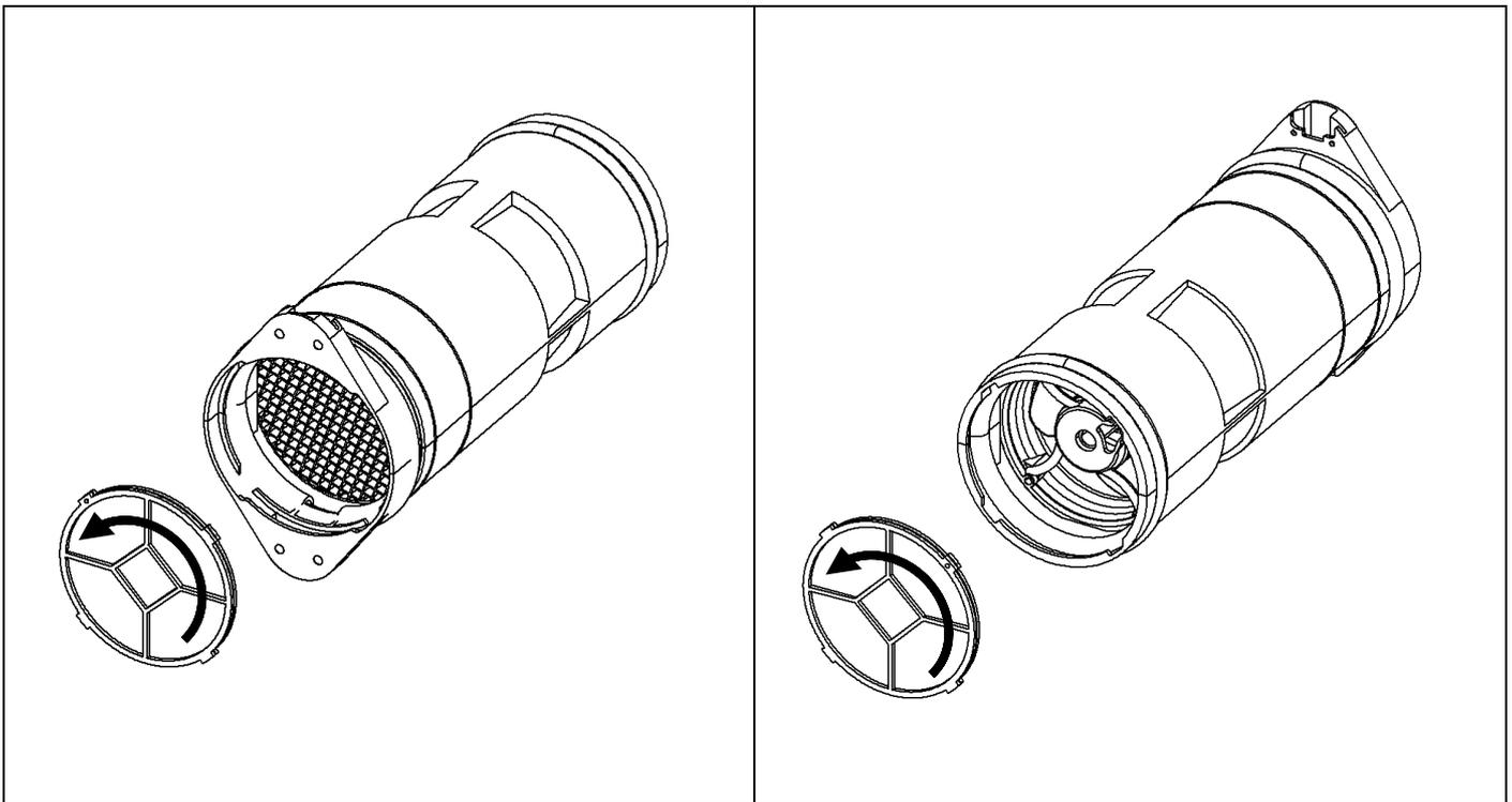
3. You can remove the filter pieces by turning them counter-clock wise and pulling them off from the capsule piece. You do not need to disassemble the capsule pieces just to remove filters.
