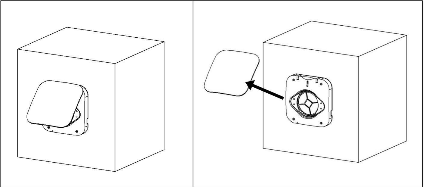
1. Remove the front cover piece by first tilting it about 45 degrees and then pulling it up from the inner cover piece.
