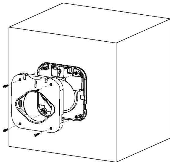
2. After making the electrical power connection mount the inner cover piece on the wall fixture part and then screw it into its place.
