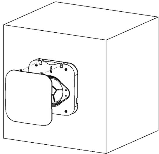
4. Put the front cover part on to the inner cover part and push the hinges. Make sure that both hinges are securely clicked in place.
