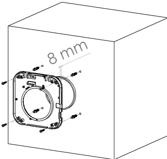
5. Align the outer wall fixture part with the 8mm protrusion of the telescopic pipe part. Drill 4 holes then insert dovels and screw the part on to the wall.
