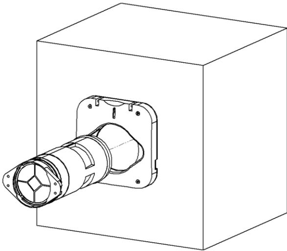
3. Align the capsule part such that the fan socket is on the left. Then push it inside the pipe, making sure the fans socket is correctly seated.
