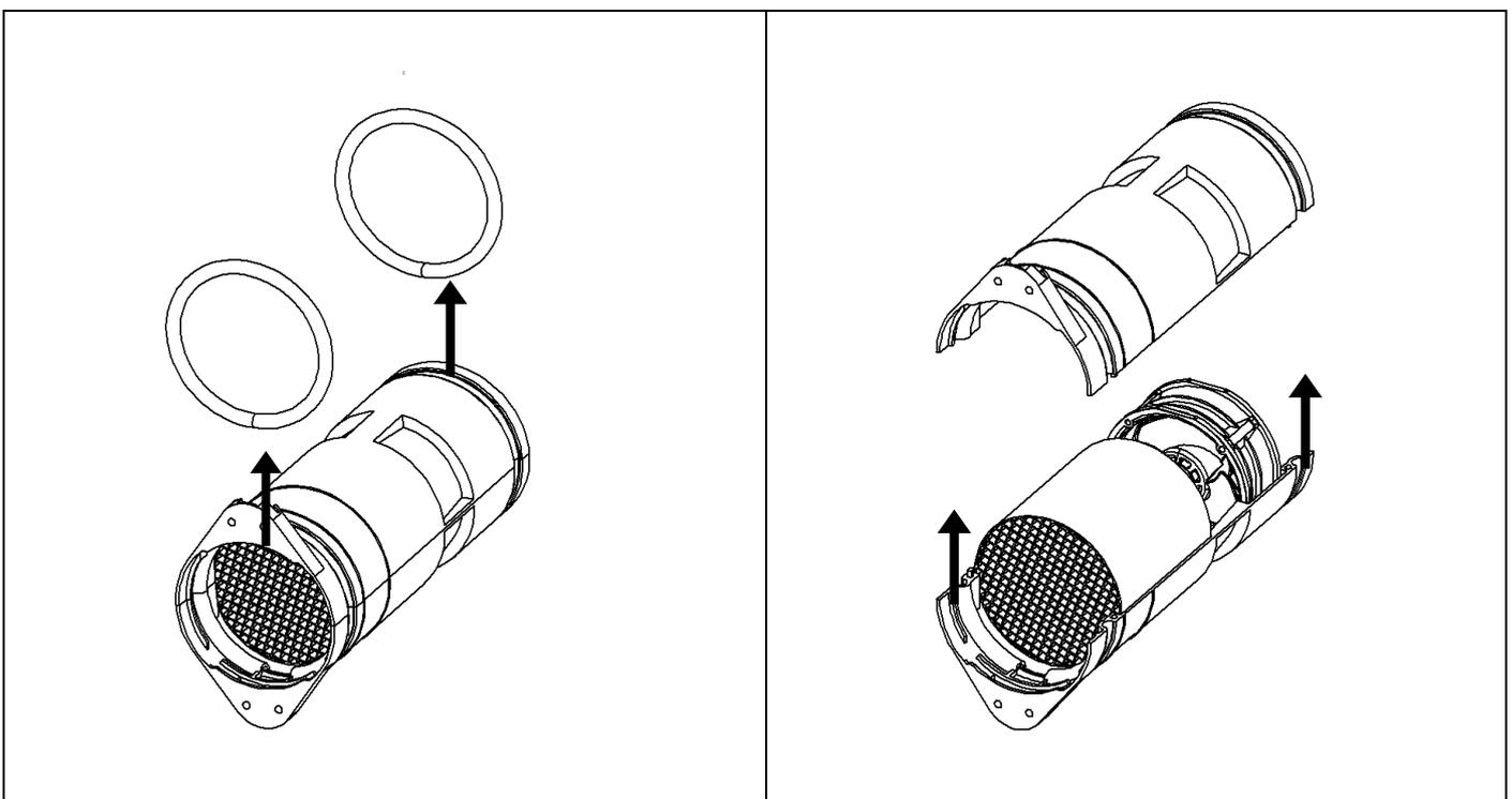
5. Remove the 2 elastic gaskets holding the capsule together. Be careful that once the gaskets are off there will be nothing holding the 2 halves of the capsule together
