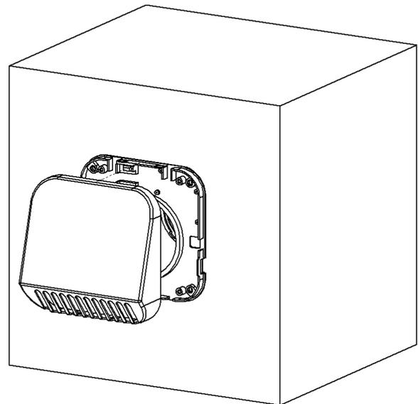
6. Place the outer hood part on to the wall fixture part and push it in its place. Make sure that the parts are securely clicked in place.
