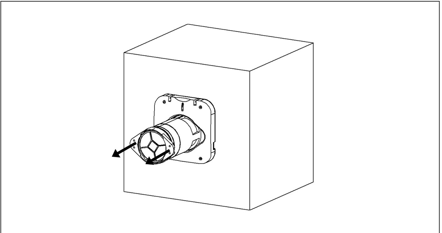
2. Remove the capsule piece by holding it from its sides and pulling it off from the pipe.
